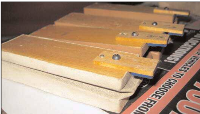
Figure 34. Secondary pneumatics prior to rebuilding.
