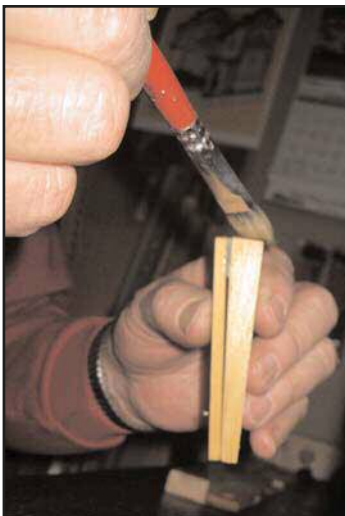
Figure 42. Applying hide glue for the outside hinge.
