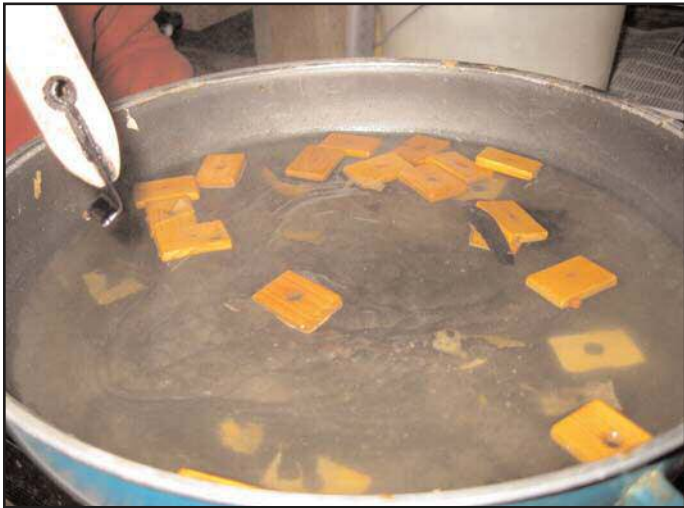
Figures 19 (above) and 20 (below). Removing leather, gaskets, and glue from primary pneumatics.
