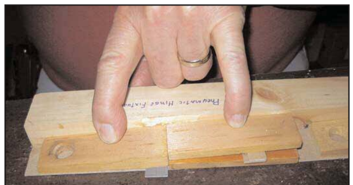
Figure 38 (below). Aligning wood blocks of secondary pneumatic.
