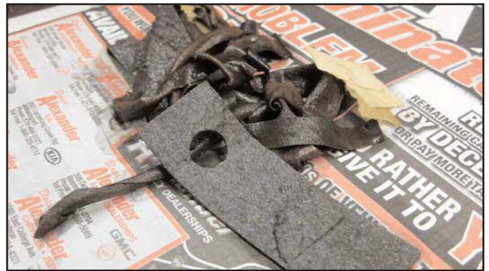
Figure 36. Leather and gaskets removed from secondary pneumatics.
