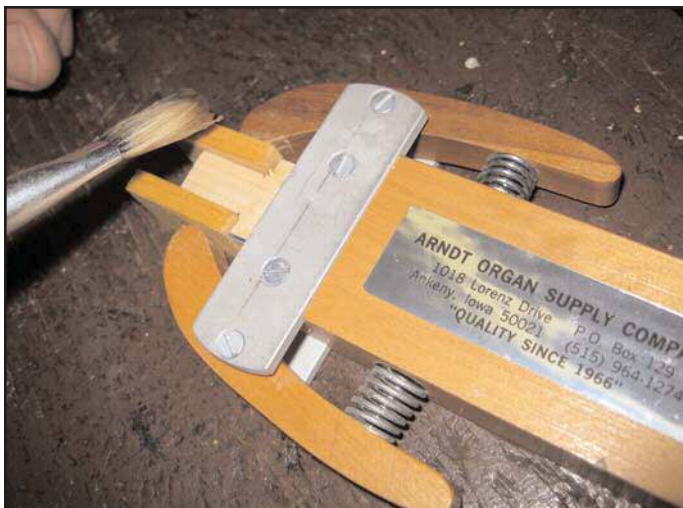
Figure 24. Clamp and custom spacer for holding primary pneumatic blocks.
