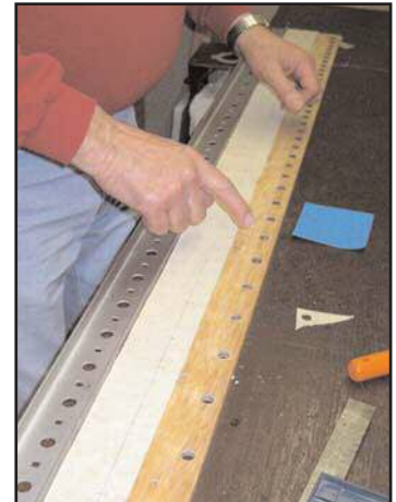
Figure 59 (above). Measuring and marking the valve cover gasket. Figure 60 (below). Punching holes in the valve cover gasket.
