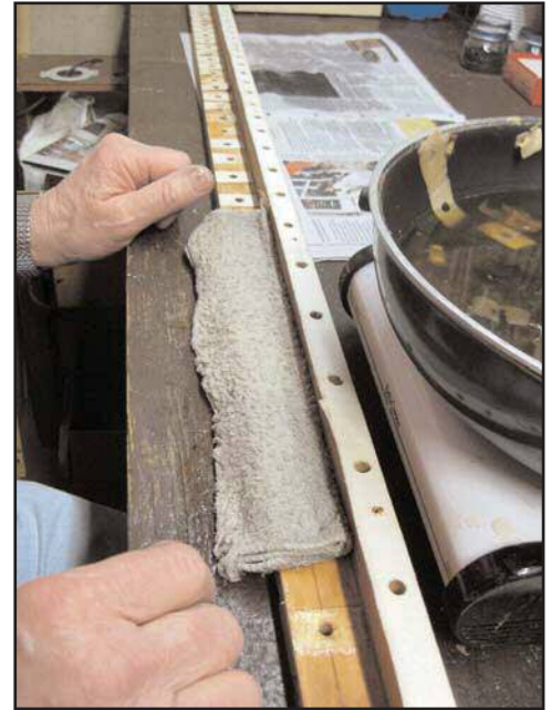
Figure 17. Removing primary pneumatic gaskets.
