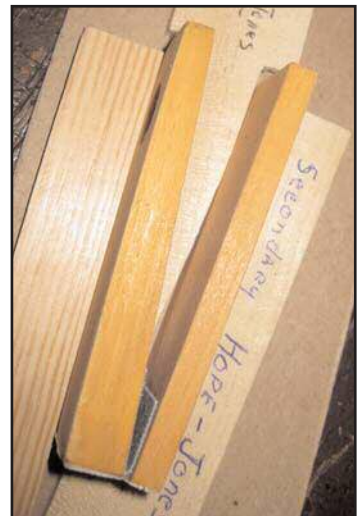
Figure 46. Secondary pneumatic placed in jig.
