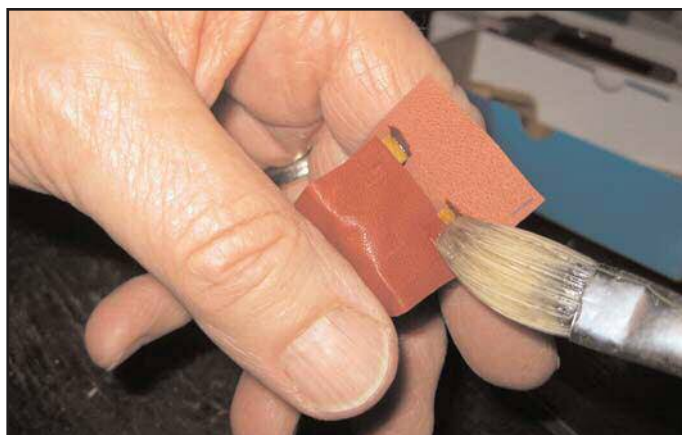
Figure 26 (top). Gluing 4th side of primary pneumatic, 1st stage Figure 27 (above). Gluing 4th side of primary pneumatic, 2nd stage. Figure 28 (below). Gluing 4th side of primary pneumatic, 3rd stage. Figure 29 (bottom). Re-leathered primary pneumatics.
