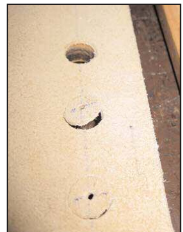
Figure 59 (above). Measuring and marking the valve cover gasket. Figure 60 (below). Punching holes in the valve cover gasket.
