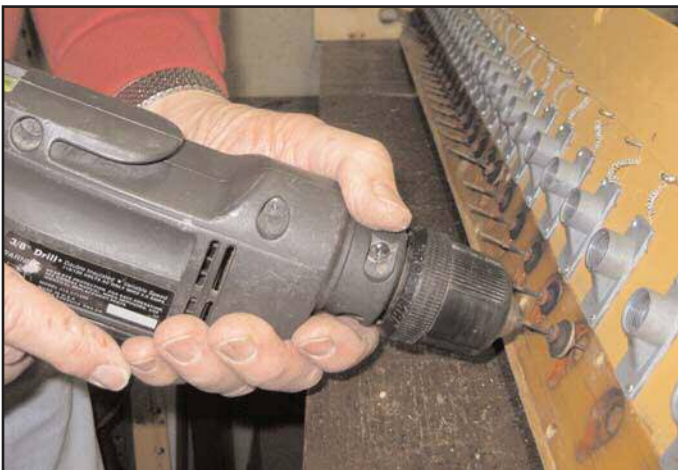
Figure 11. Removing primary valves with a keyless chuck drill.
