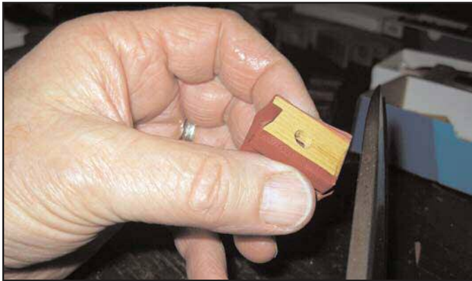
Figure 30. Trimming the leather on primary pneumatics.
