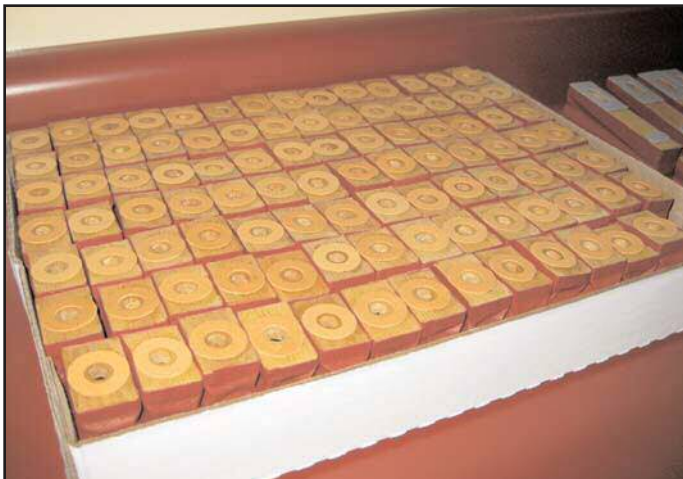
Figure 31. Rebuilt primary pneumatics.
