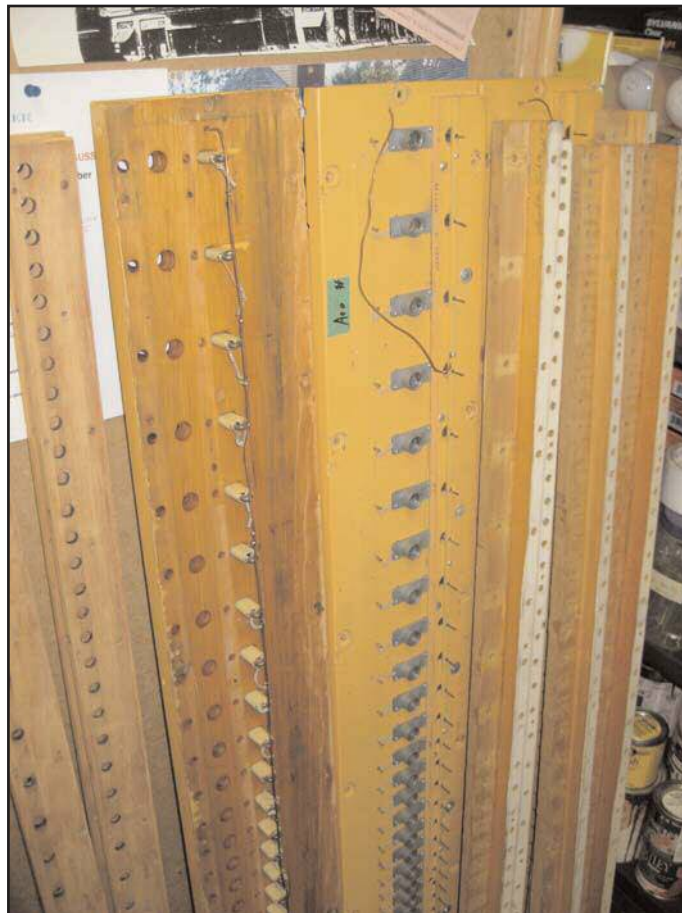
Figure 9. The pipe chest bottom boards.
