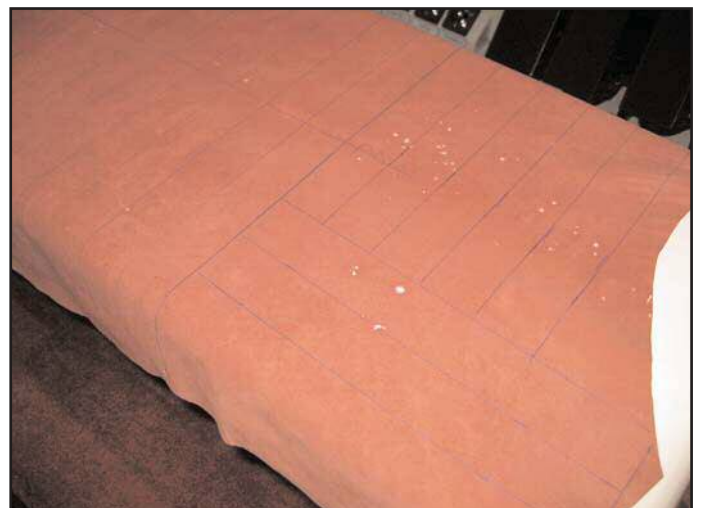
Figure 23. Leather hide marked for cutting.
