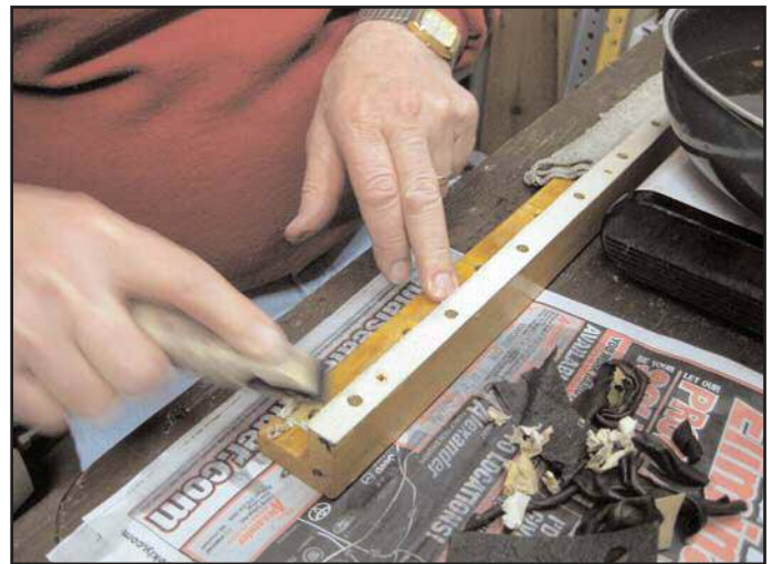
Figure 18. Removing primary pneumatic gaskets and glue.
