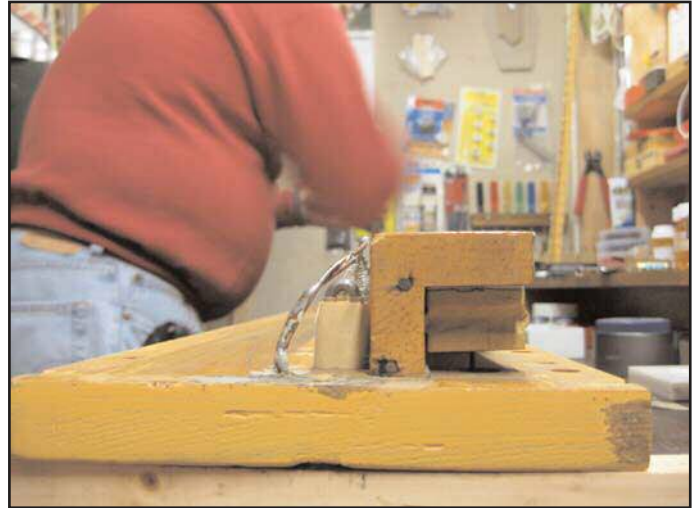
Figure 12 (above). Bottom board with magnets, primary rail and primary pneumatics.
