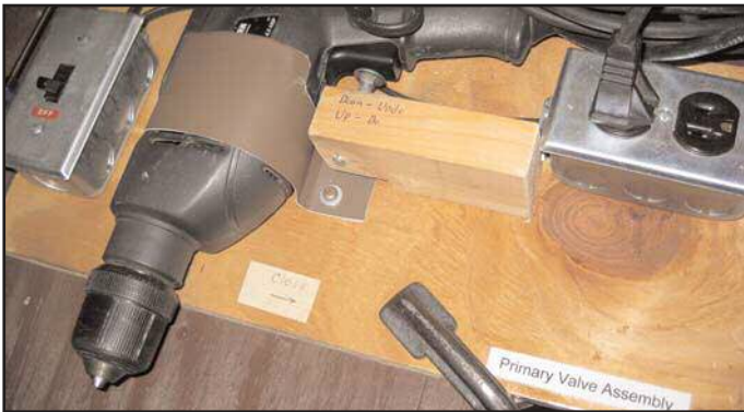
Figure 56 (above). Drill jig for threading nuts onto valve wires.
