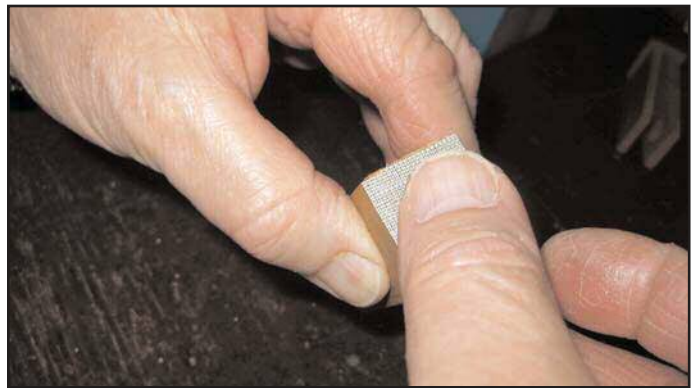
Figure 43. Applying hide glue for outside hinge (different view). Figure 44 (below). Applying muslin for outside hinge. Figure 45 (bottom). Outside hinges of secondary pneumatics drying.
