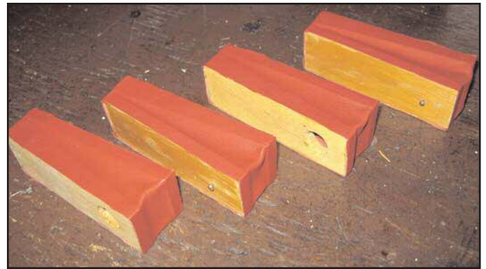
Figure 52. Re-leathered secondary pneumatics drying
