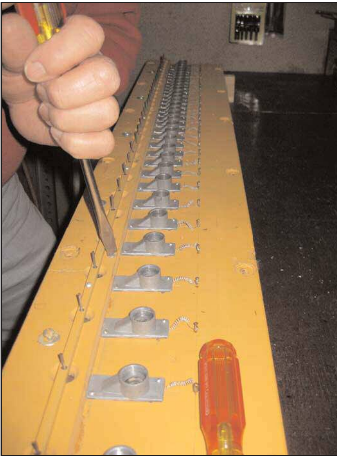
Figure 10. Removing the valve cover from the bottom board.
