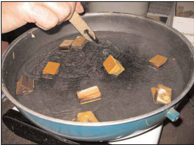
Figures 19 (above) and 20 (below). Removing leather, gaskets, and glue from primary pneumatics.
