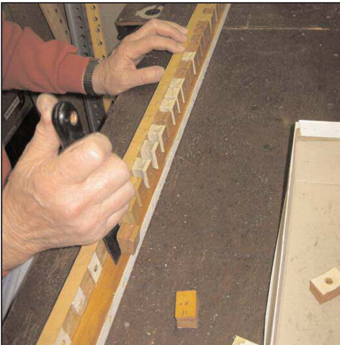
Figure 16. Separating the primary pneumatics with a putty knife.
